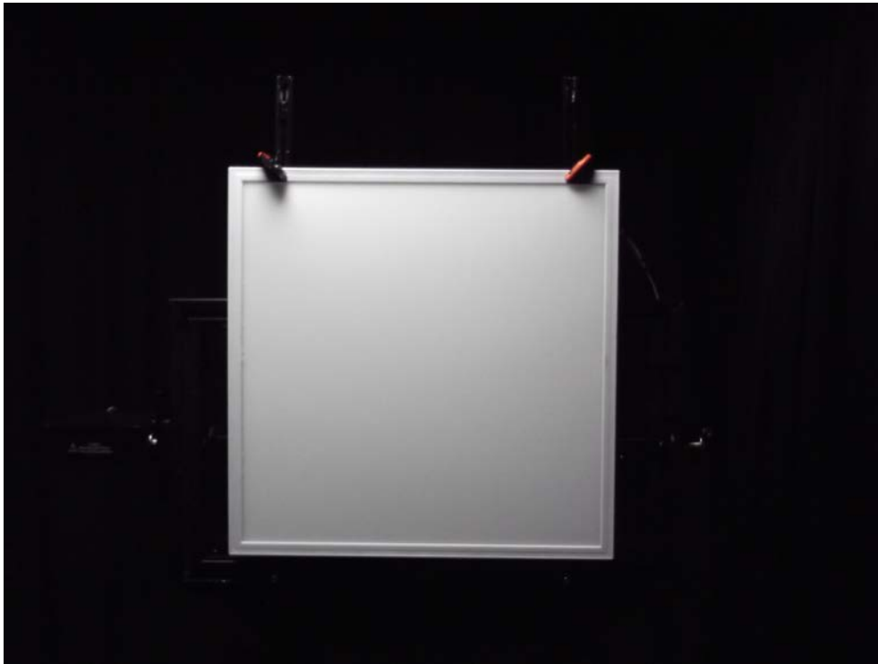
Photo 1: Luminaire on goniometer mount
